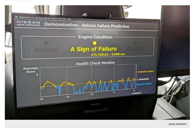
Researchers from Nissan Motor Co., and Canadian tech firm Acerta Analytics Solutions Inc. are putting a new artificial intelligence tool designed to predict engine component failures through its paces.
